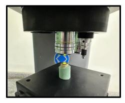
Figure (2) Dentin sample on Vickers microhardness testing machine
