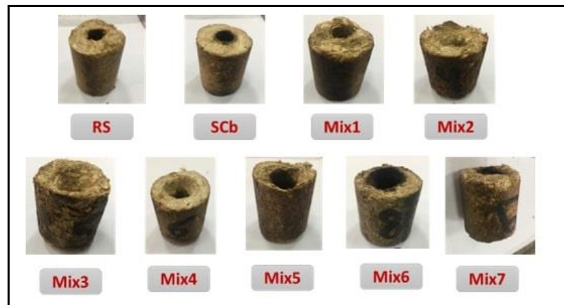
Fig. (5): Briquettes samples made from agricultural residues mixtures (rice straw (RS), sugar cane bagasse (SCb), banana peels, coconut shell, cattle manure) using a screw press.
