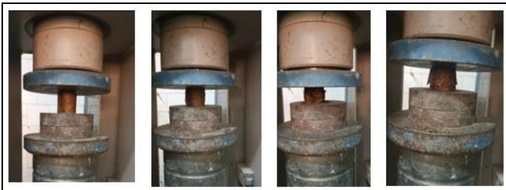
Fig. (9): Compressive stress test until briquettes failure.
