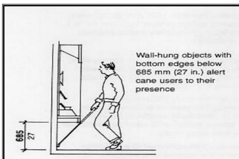
Fig.44. Cane detection of wall hung case, (Majewski, J. Part of Your General Public Is Disabled . PP. 229-293)
