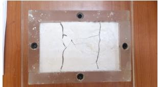
Figure 8 Crack appearances in gelled ceramics
