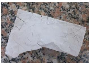
Figure 10 Improper surface cracks
