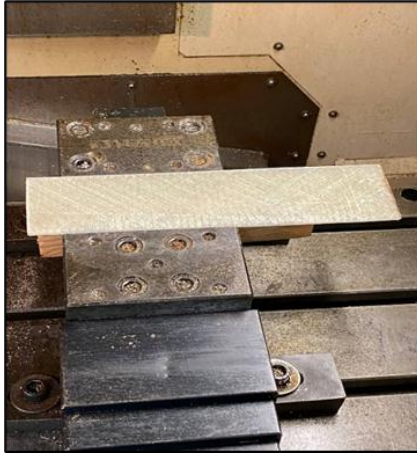
Figure 1: Fixing of a GFRP composite plate.
