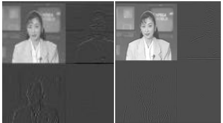
Fig2: An example of lifting wavelet decomposition (left) and stationary wavelet decomposition (right).
