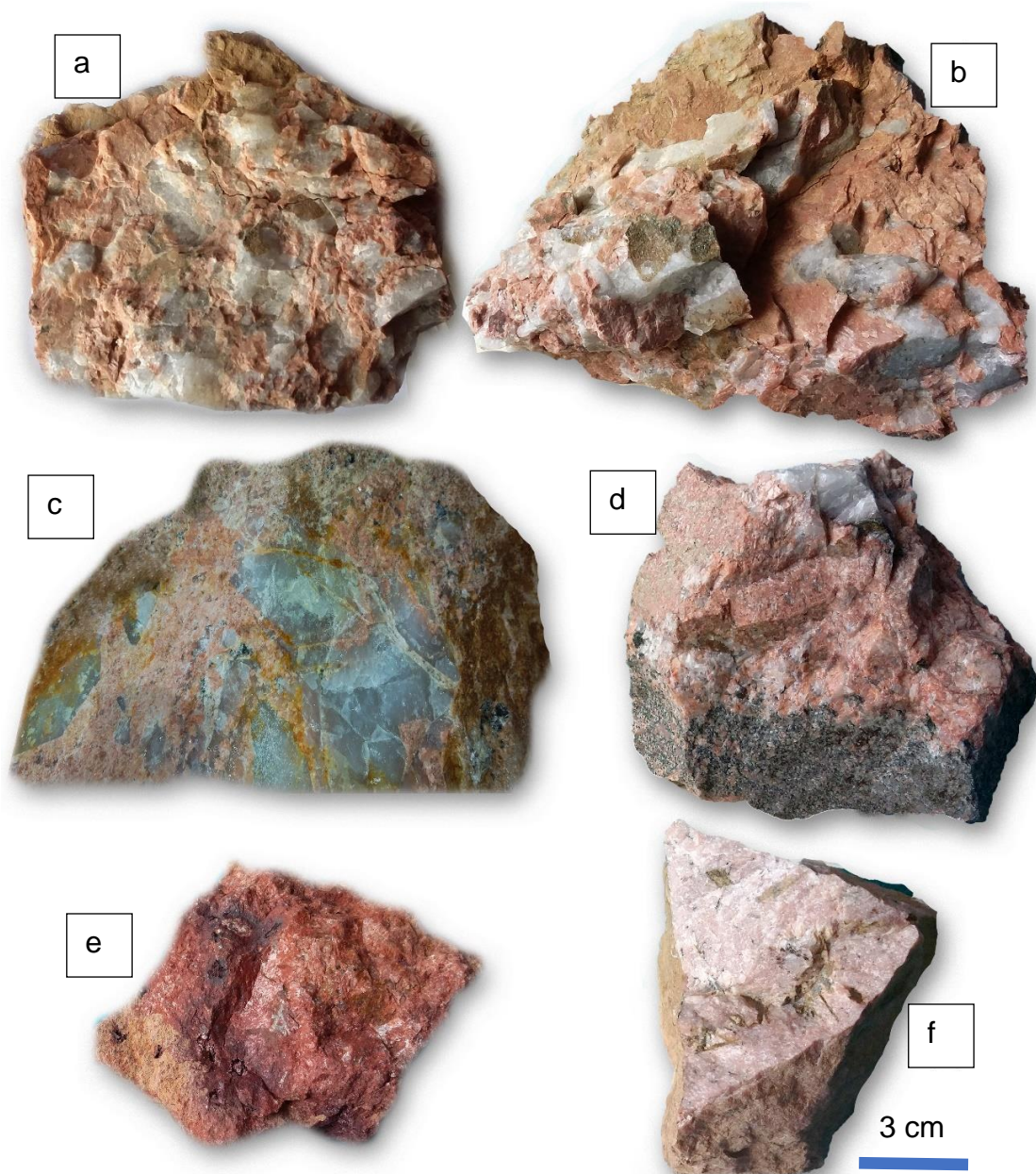
Plate 1: Characteristic features of hand specimens of Wadi Ghadir pegmatites, a) Quartz crystals within K-feldspar; b) and c) Variable K-feldspars/ quartz ratio; d) K-feldspar in wall zone; e) Brick-red K-feldspar, intermediate zone; f) Rose color quartz, core zone.
