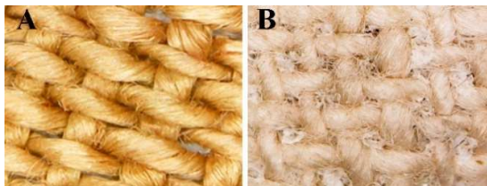
Figure 3: Shows the weaving structure of both the artifact (A) and the experimental piece (B) at a magnification of 10X
