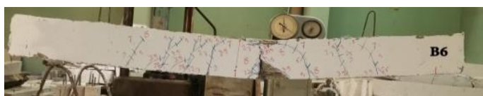
Fig. 9 Pattern of cracks of beam (W).
