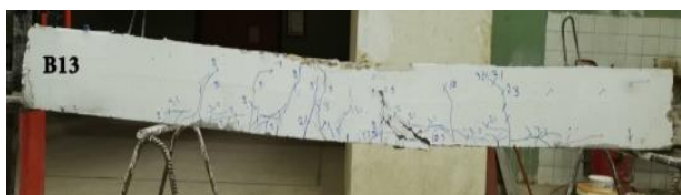
Fig. 12 Pattern of cracks of beam (W3).
