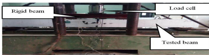
Fig. 5-A Set up of tested beams
