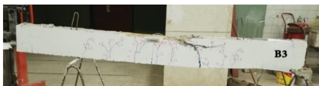
Fig. 8 Pattern of cracks of beam (G1).
