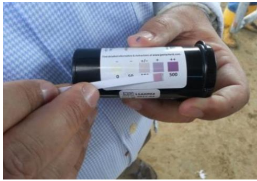
Figure 2 the change in the color of PortaBHB milk ketone test strips on milk samples.
