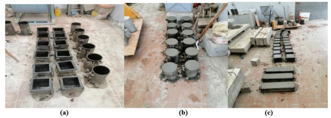
Fig 2. Test specimens: (a) Forms, (b) cylinders and (c) cubes and beam specimens
