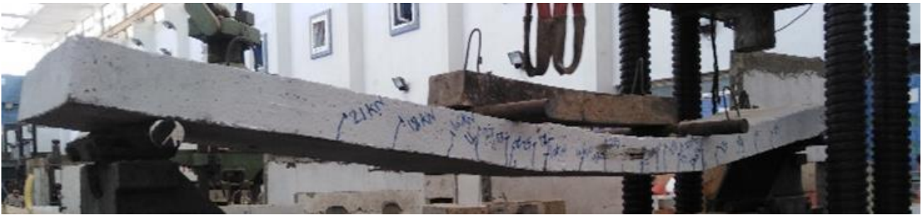
Fig. 8: Crack pattern for RC slab, S-St-Control
