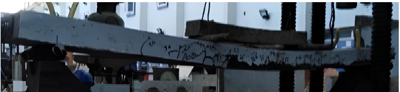
Fig. 11: Crack pattern for RC slab, S-BF-50%-Int.
