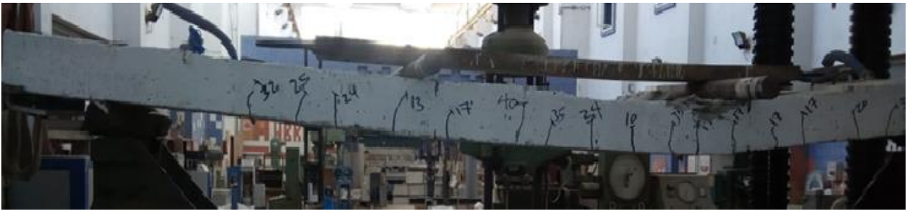
Fig. 13: Crack pattern for RC slab, S-St-BF-10%-Ext.
