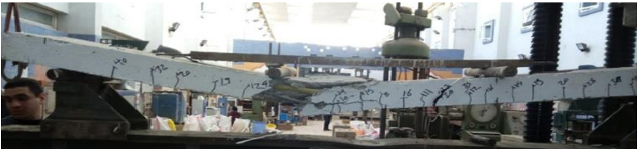
Fig. 14: Crack pattern for RC slab, S-St-BF-30%-Ext.
