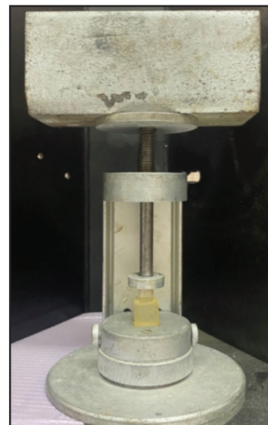
Fig. (5) A specially designed device used to standardize load during bonding
