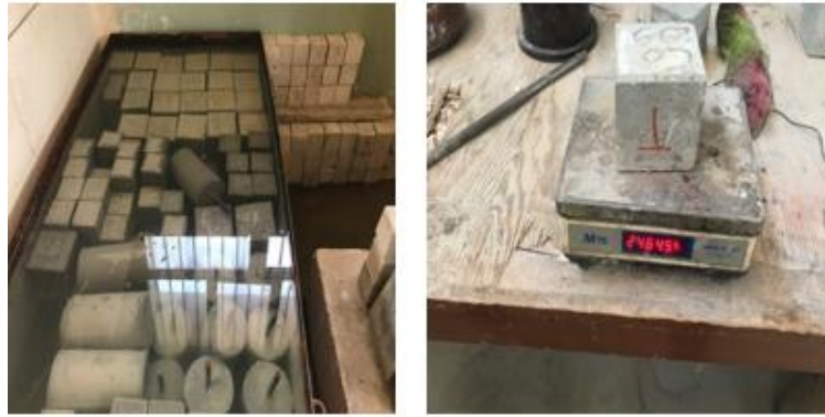
Fig. (6): Partial water absorption test.
