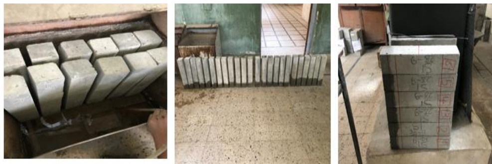
Fig. (8): Capillary water absorption test.
