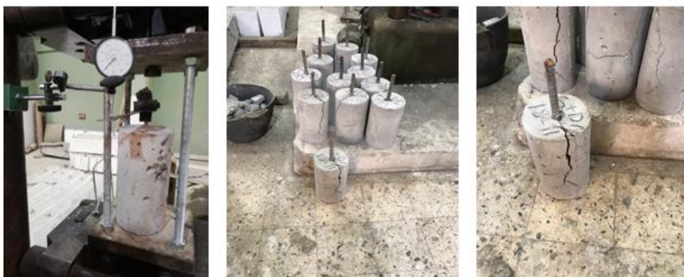
Fig (5) Shape of bond failure of concrete specimens.
