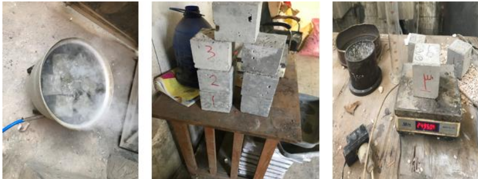
Fig. (7): Total water absorption test.
