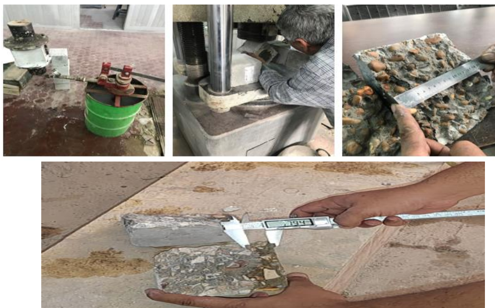
Fig. (9): Water Penetration test.
