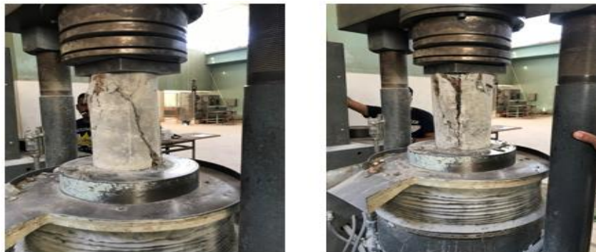
Fig (3): Digital universal testing machine capacity 150 ton for testing cubes and cylinders.
