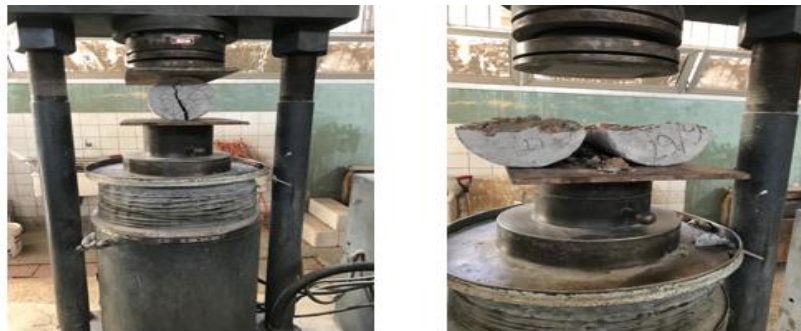
Fig (4): Splitting tensile stress test.
