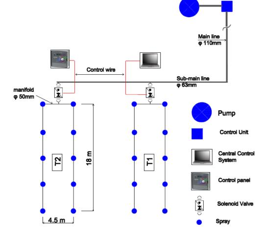
Fig. 1. Experimental Layout.
