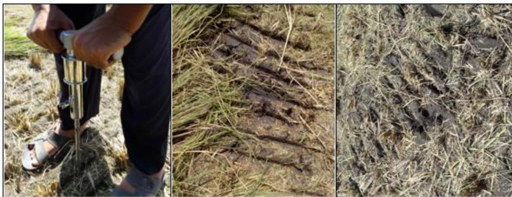
Fig. 1. Measuring soil penetration resistance and print sinkage of the combine crawlers.
