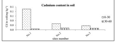
Fig, 5: Effect of fly ash on AB-DTPA Cadmium content in different soils depth and sires. Sites No.1= El-Alban area, 2= El-Nagagra area and 3= El-Shatb area.
