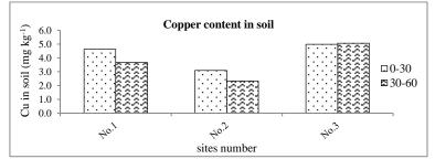
Fig, 4: Effect of fly ash on AB-DTPA Copper content in different soils depth and sires. Sites No.1= El-Alban area, 2= El-Nagagra area and 3= El-Shatb area.
