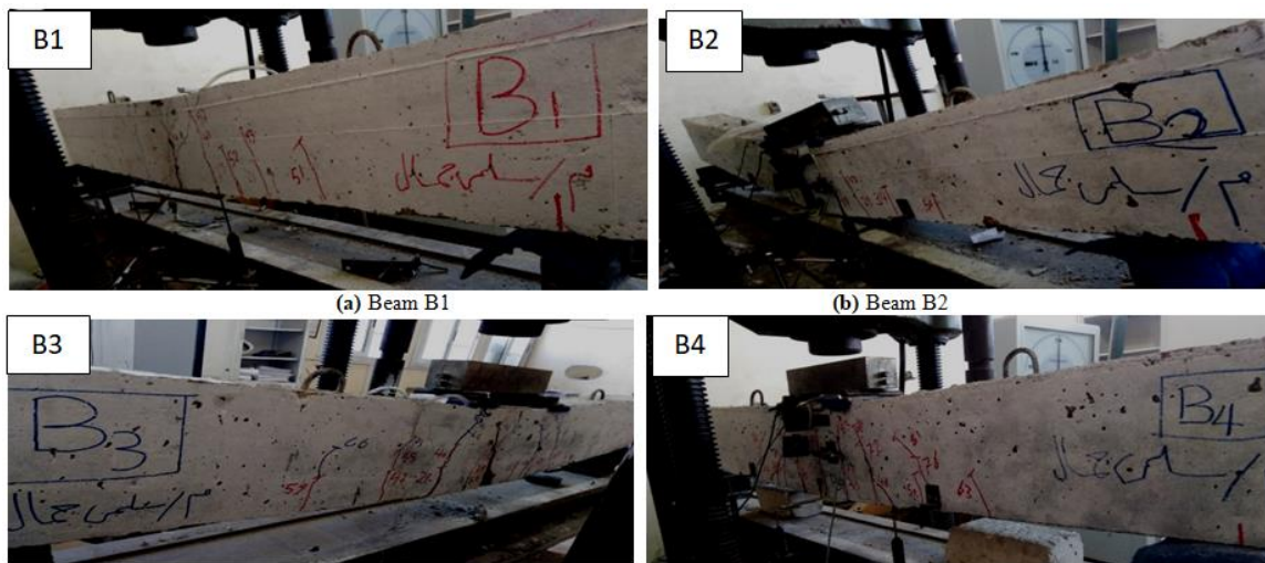
Fig 12. Crack patterns for beams of Group I (reinforced by steel bars).
