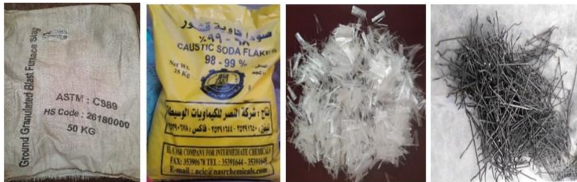
Fig 1. Geopolymer constituent materials and added fibers.
