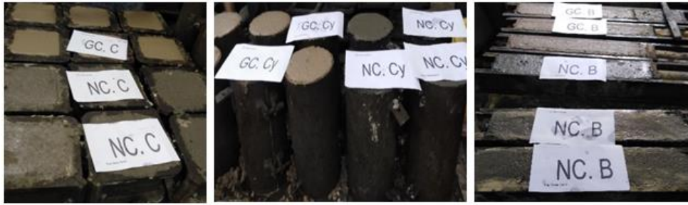
Fig 5. Test specimens for normal and geopolymer concrete mixes.
