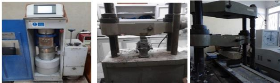
Fig 6. Compressive, splitting tensile and flexural tests for concrete specimens.
