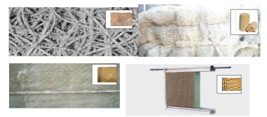
Fig. 3. Types of the evaporative cooling pads in the greenhouse
