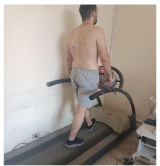
Figure 1: EMG set up for GMax and LD muscles during treadmill walking
