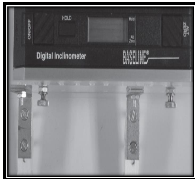
Figure (1): Modified digital inclinometer
