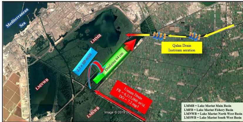
Fig. 8. Illustrate the instream aeration before the dilution of Qalaa Drain waters with Umum Drain waters to improve the water quality of Qalaa Drain.
