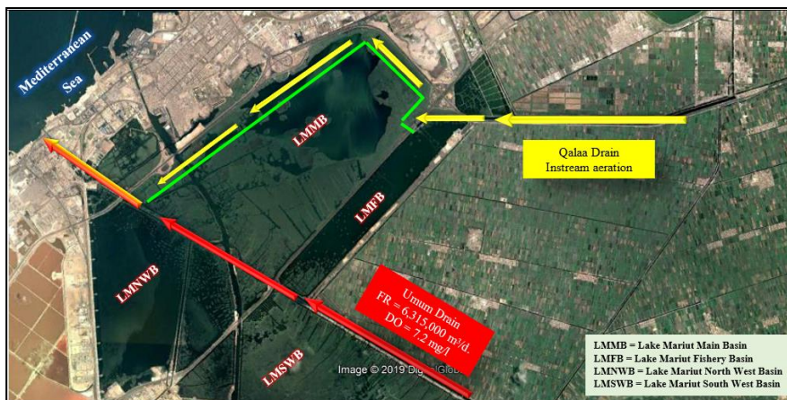
Fig. 9. Illustrate the solution by diversion of polluted Qalaa Drain waters from Lake Mariut Main Basin to improve the water quality of the basin.
