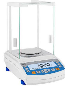
Fig. 1 Universal friction and wear testing machine. Fig. 2 Balance 10^{-4} grams resolution.
