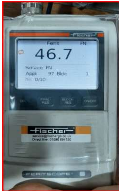
Fig. 5 Ferrite percentage content during measurement by using a ferrite-scope.
