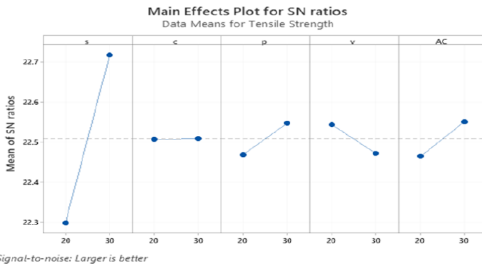
Fig. (9): Main effects plot of SN ratios for tensile strength using the Taguchi method
