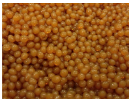
Fig. (3): Optical photograph of CuF/NBR beads.
