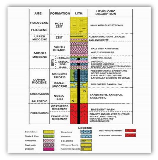
Fig. (5): Generalized stratigraphic column of Zeit Bay field (after SUCO,1988)
