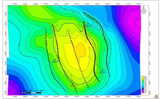
Fig. (7): Depth structure contour map on top Rudies in Zeit Bay field.
