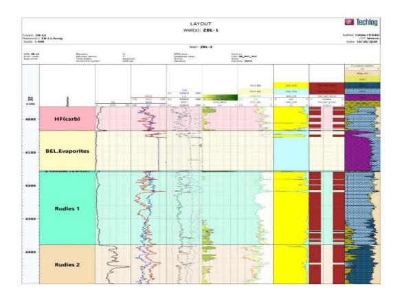
Fig. (11): Computer processed interpretation (CPI) of ZB-L1 well by Techlog program software.
