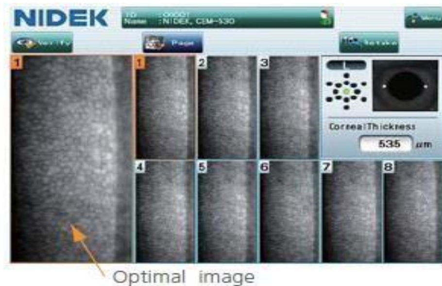
Fig. (2): CEM-530 specular microscope captures 16 images auto indication of the optimal image with orange highlight.
