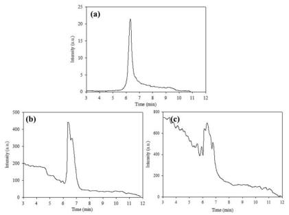
Fig. 1. Chromatogram of the standard PC (a), hen egg yolk phospholipids (b), duck egg yolk phospholipids and (c) (Mobile phase, methanol; flow rate, 1.0 ml·min<sup>-1</sup>; column temperature, 30 °C; sample injection, 10, 20 and 40 μl, respectively).
