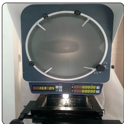
Fig. (1) Contact angle analysis using a vertical profile projector.
