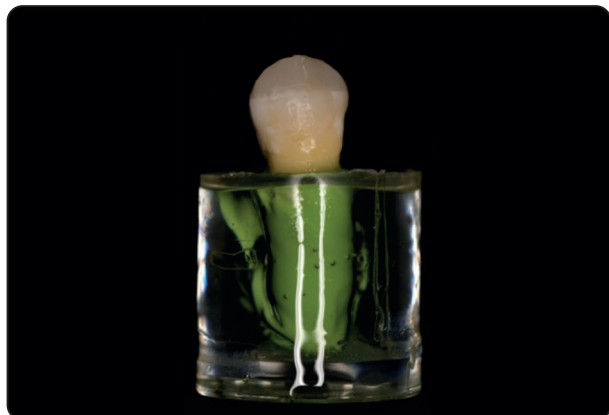
Fig. (1) A tooth mounted in epoxy resin mold with periodontal ligament simulation.
