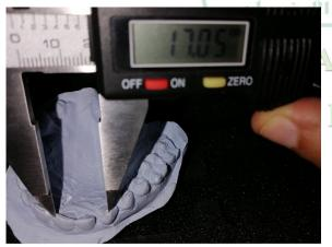
Figure 4 - Using caliper for measuring 1Rt-2Rt distance
