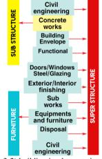
(Figure 3-2) building implementation phases Source: Adapted by the researcher based many observation for implemented projects in Egypt
