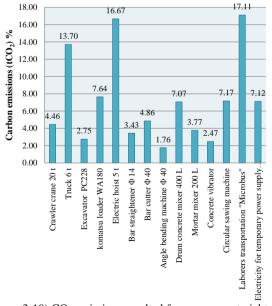
(Figure 3-10) CO<sub>2</sub> emissions resulted from every material type during its construction phase
