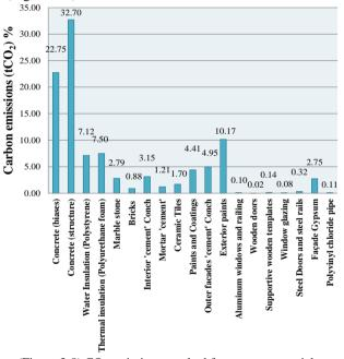
(Figure 3-8) CO<sub>2</sub> emissions resulted from every material type during its preparation phase
