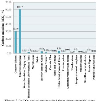
(Figure 3-9) CO<sub>2</sub> emissions resulted from every material type during its transportation phase
