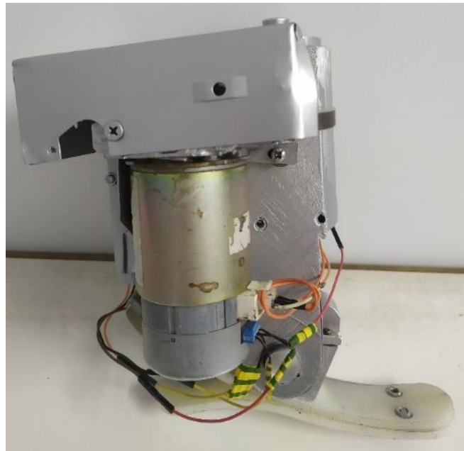
Fig. 22: the semi-active ankle prosthesis.
