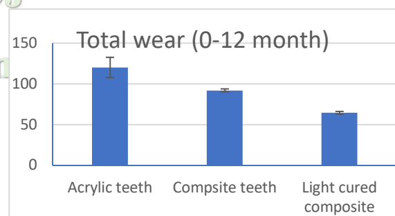
Fig (5) Bar graph comparing total wear of different denture teeth materials during 0-12 months interval
