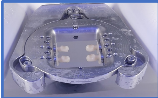
Fig (6): Milled crowns fixated in milling machine
