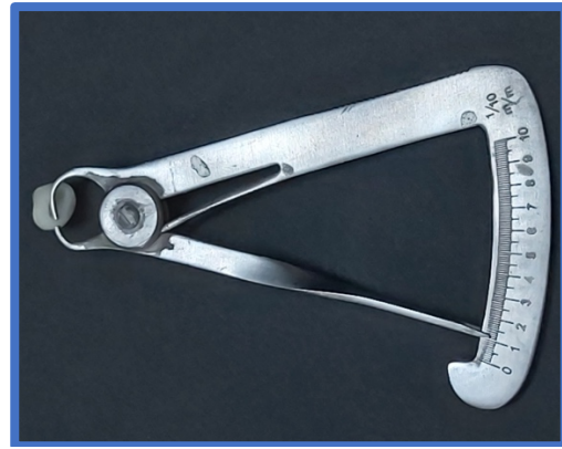
Fig (8): checking marginal thickness using manual caliper
