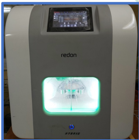
Fig (7): milling machine (Redon Hybrid machine)
