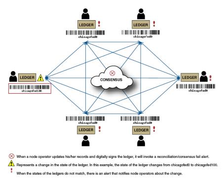
Figure3. Disbursed ledger (DL) network channel-New record added and state changes
