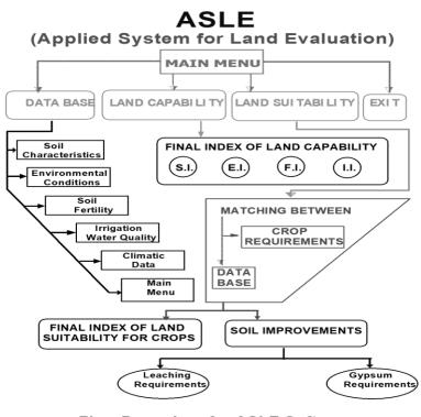
Flow Procedure for ASLE Software. Fig. 2. Flow chart ASLE- program.
