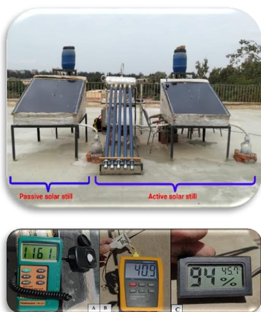
Fig. 1. The experimental design and placement of sensors arrangements of active and passive solar still.
