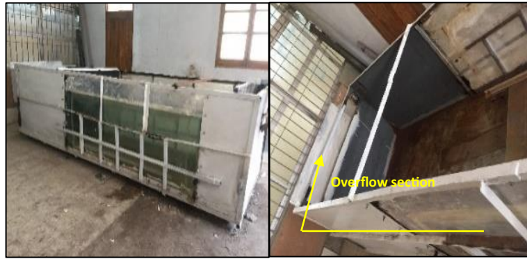
Fig. 3: Wave basin and the overflow section (field photo)
