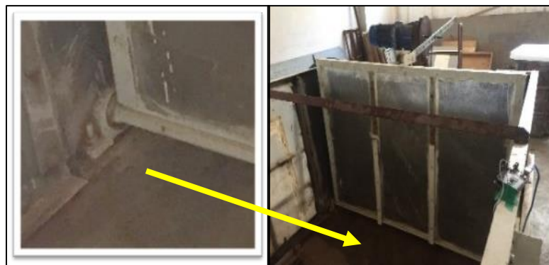
Fig. 2: Wave generator with its supporting system
