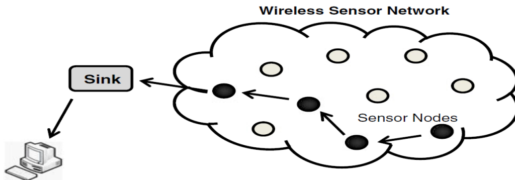
Fig. 1: Collection of data in a scenario of a wireless sensor network [29].
