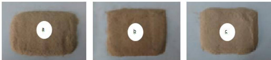
Fig. 2: Chitosan extracted from shrimp shells by different techniques; a- traditional technique, b- microwave technique and c- by autoclave technique.
