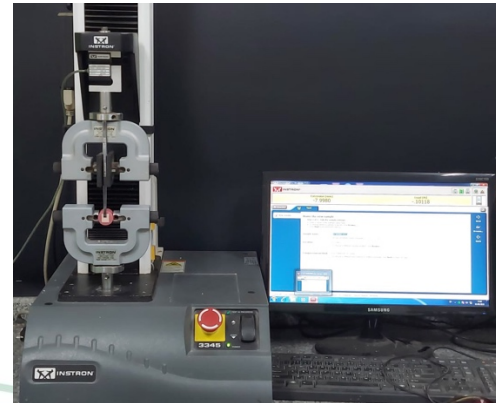
Figure 6: Universal test machine for shear bond strength
