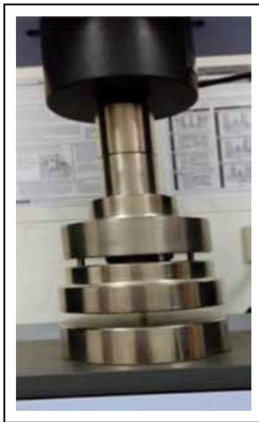
Fig. (2): Universal testing machine used for compressive strength testing
