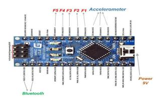
Figure .6. Arduino Nano and its peripherals connections.
