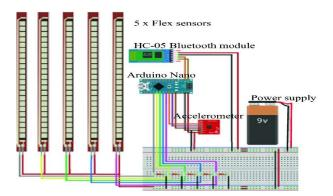
Figure .5. SSG Circuit diagram.
