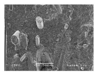
Fig .4 SEM micrograph of fracture surface of date palm fibre/polyester composite[54]
