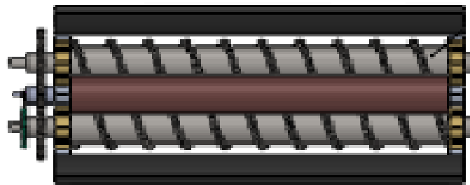
Fig. (5) - Plan of the husking unit cylinders in machine for showing the clearance between the two husking cylinders surfaces.
