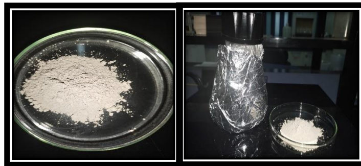
Fig .4. kaolin powder that used in this search Prepared at Temperatures 103-105°C.
