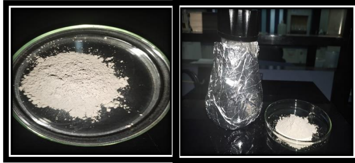
Fig .2. kaolin powder that used in this search Prepared at Temperatures 103-105°C.
