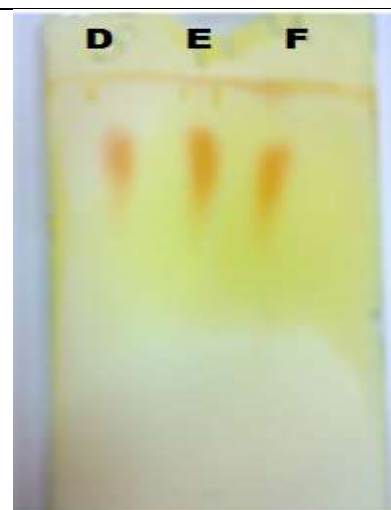
Figure 4b: TLC for THC before adulteration of THC positive sample, D. after adding Clorox, E. after water dilution, F. THC standard from right to left. Silica gel plates spraying with acidified Fast Blue
